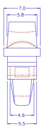
© HOLE IN CHASSIS: Ø4.8
