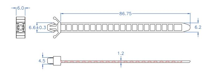
© HOLE IN CHASSIS: Ø5.0
