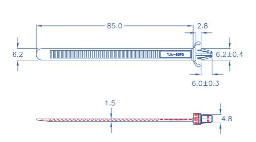
© HOLE IN CHASSIS: Ø5.0
