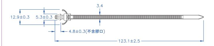
O HOLE IN CHASSIS: Ø4.0
