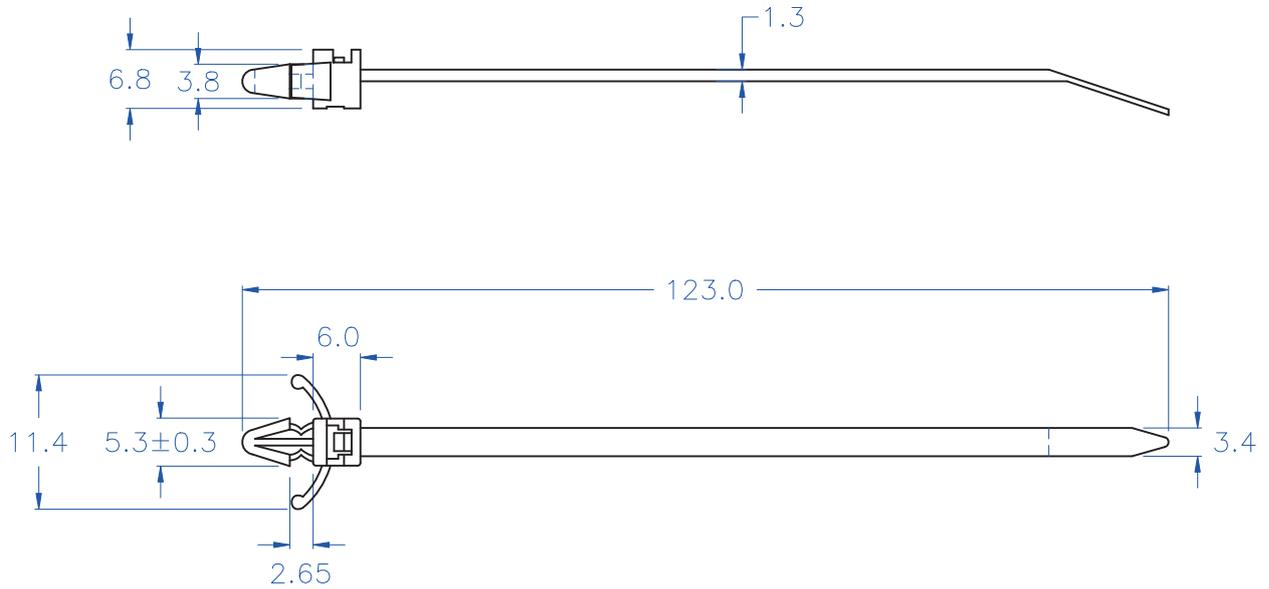
◎ HOLE IN CHASSIS:  $\phi 4.0^{+0.05}_0$  mm
