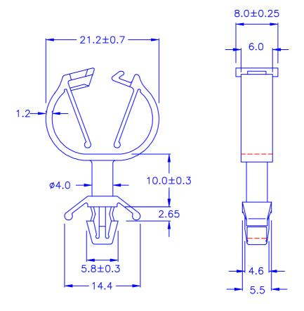
○ HOLE IN CHASSIS: Ø4.8~Ø5.0mm
