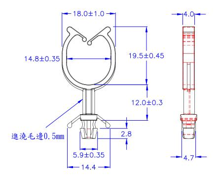
© CHASSIS THICKNESS: 0.5~2.3 mm © HOLE IN DIMENSIONS: Ø4.8~Ø5.0
