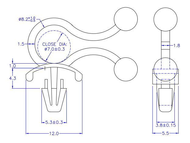
O HOLE IN CHASSIS: Ø4.0
