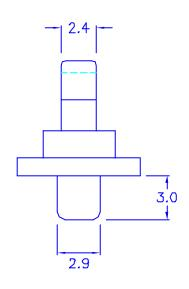
© CHASSIS THICKNESS: 0.8 mm © HOLE IN DIMENSIONS: Ø3.0
