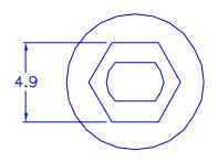
© CHASSIS THICKNESS: 1.6 mm © HOLE IN DIMENSIONS: Ø3.2
