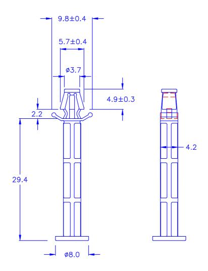
O HOLE IN CHASSIS: Ø4.0
