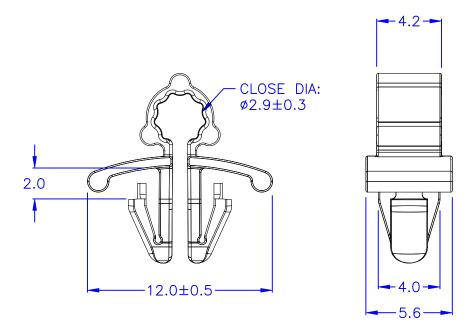
© HOLE IN CHASSIS: Ø4.5
