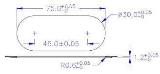
$\bigcirc$  CHASSIS THICKNESS: 1.2 $^{+0}_{-0.05}$  mm
