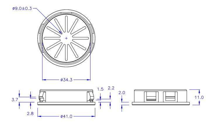
© HOLE IN DIMENSIONS: Ø38.1 +0.1 © CHASSIS THICKNESS: 1.2~3.2 mm
