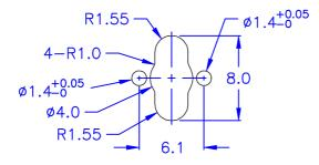
$\bigcirc$  CHASSIS THICKNESS: 1.6 $^{+0}_{-0.05}$  mm
