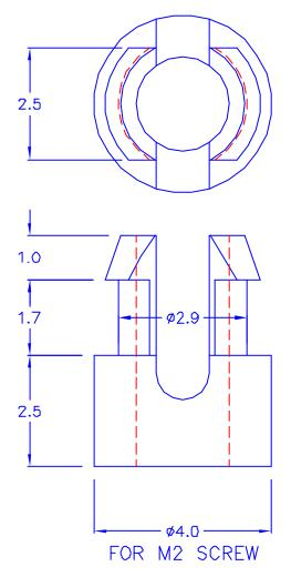
© P.C.B THICKNESS: 1.6 mm O HOLE IN DIMENSIONS: Ø3.0
