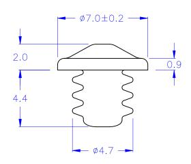
○ HOLE IN CHASSIS: Ø4.1±0.1 mm
