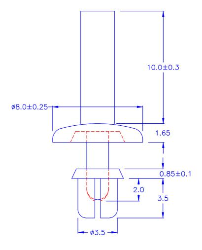
O HOLE IN CHASSIS: Ø3.5
