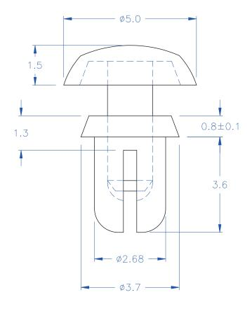
$\bigcirc$  HOLE IN CHASSIS:  $\emptyset 2.7^{+0.05}_{-0}$  mm © CHASSIS THICKNESS: 1.0~2.0 mm
