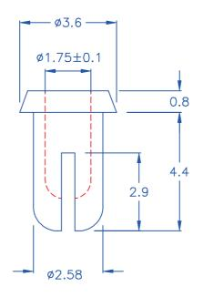
© HOLE IN CHASSIS: Ø2.6
