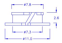
© CHASSIS THICKNESS: 1.1 mm © HOLE IN DIMENSIONS: Ø7.24
