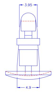
© HOLE IN CHASSIS: Ø5.5
