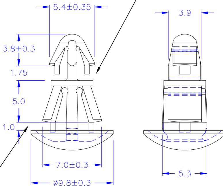
◎ HOLE IN P.C.B.:  $\phi 5.5^{+0.05}_0$  mm
