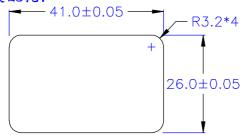
© THICKNESS: 0.8 mm ◎ 閉合尺寸須裝人裝配孔後量測
