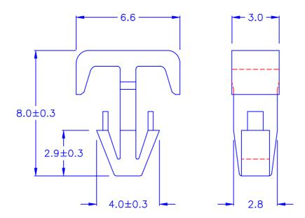
© HOLE IN CHASSIS: Ø3.0
