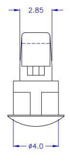
O HOLE IN CHASSIS: Ø3.0
