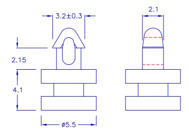
© CHASSIS THICKNESS: 2.0 mm © HOLE IN DIMENSIONS: Ø2.5
