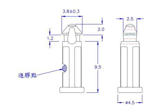
© HOLE IN P.C.B.: Ø3.0 mm ◎ P.C.B. THICKNESS: 0.8~1.0 mm
