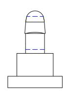
© HOLE IN DIMENSIONS: Ø2.0 © CHASSIS THICKNESS: 1.6 mm
