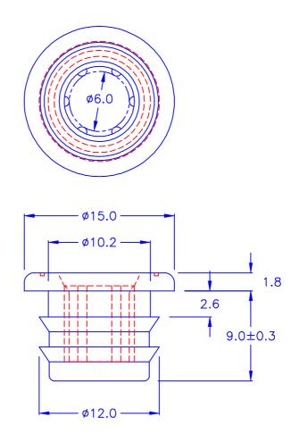
© CHASSIS THICKNESS: 2.5 mm © HOLE IN DIMENSIONS: Ø10.0
