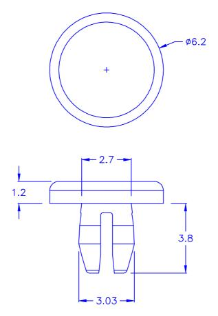
◎ P.C.B THICKNESS: >4.0 mm O HOLE IN DIMENSIONS: Ø2.8
