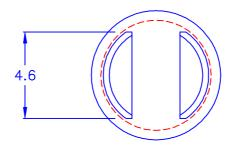
O HOLE IN CHASSIS: Ø5.0
