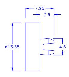
O HOLE IN CHASSIS: Ø4.3
