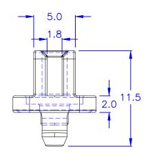
OHOLE IN CHASSIS: Ø3.4 mm © CHASSIS THICKNESS: 2.0 mm
