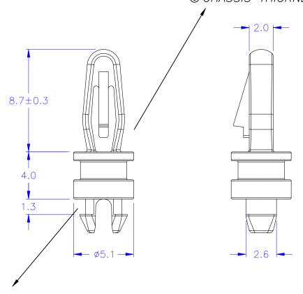
$\bigcirc$  HOLE IN CHASSIS: Ø3.2 $^{+0.05}_{-0}$  mm  $\bigcirc$  CHASSIS THICKNESS: 1.0 $^{+0.2}_{-0}$  mm
