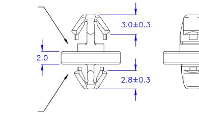
O HOLE IN CHASSIS: Ø3.8
