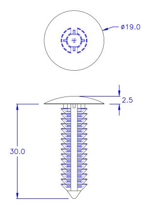
O HOLE IN CHASSIS: Ø7.1
