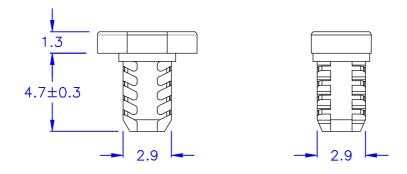
○ HOLE IN FAN: Ø3.5 +0.05 mm
