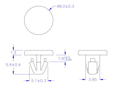
$\bigcirc$  HOLE IN CHASSIS:  $\emptyset 4.1^{+0.05}_{-0}$  mm
