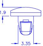
◎ HOLE IN CHASSIS: Ø3.5
