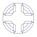
© HOLE IN CHASSIS: Ø6.5
