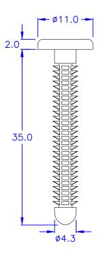
◎ HOLE IN CHASSIS: Ø4.7~Ø4.9
