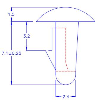
© HOLE IN CHASSIS: Ø3.2~Ø3.3
