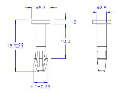
◎ HOLE IN CHASSIS: Ø3.2
