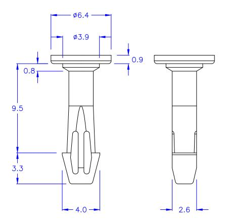
© HOLE IN CHASSIS: Ø3.0
