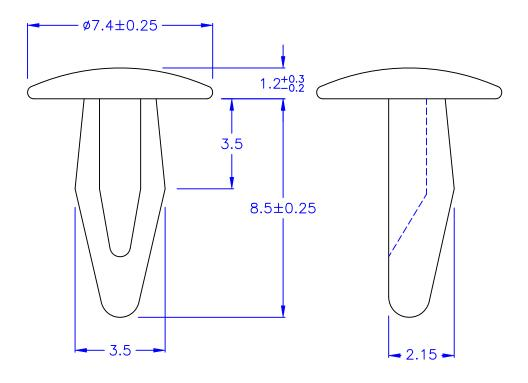
○ HOLE IN CHASSIS: Ø3.0~Ø3.2
