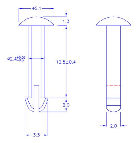
© CHASSIS THICKNESS: 10.1 mm © HOLE IN DIMENSIONS: Ø2.54
