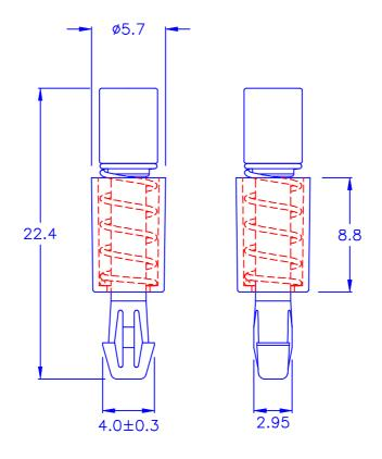
O HOLE IN CHASSIS: Ø3.0
