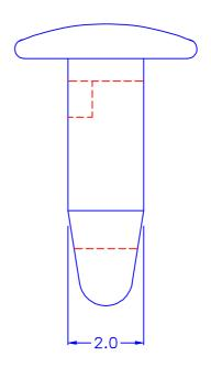
© HOLE IN CHASSIS: Ø2.37
