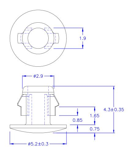
$\bigcirc$  HOLE IN CHASSIS:  $\emptyset 3.0 \sim \emptyset 3.1$  $\bigcirc$  CHASSIS THICKNESS:  $1.4 \sim 1.6$
