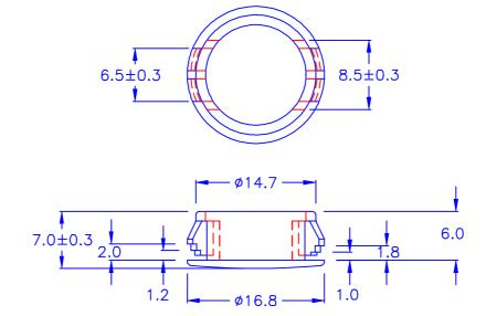
HOLE IN CHASSIS: Ø15.0~Ø15.1
